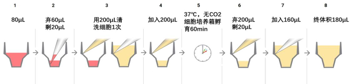
**B-Figure 3.5** 103592-100和103344-100细胞换液流程
